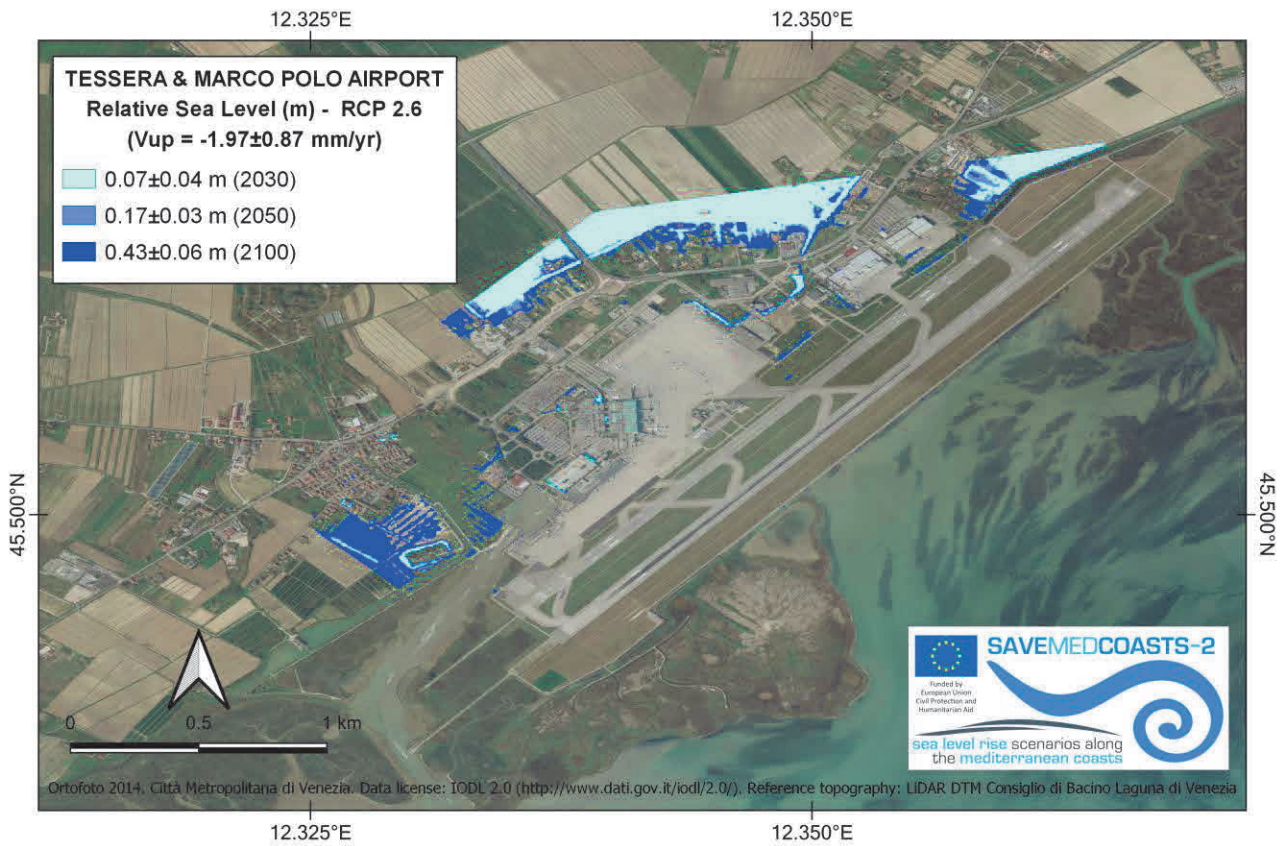
Figure 41 – The Venice lagoon: RCP 2.6 scenario of RSL at Tesserà & Marco Polo Airport.
